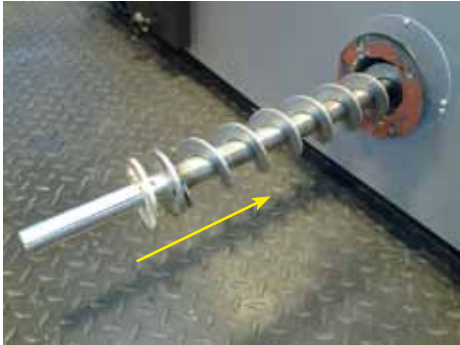
Push the primary ash screw inside the boiler.
