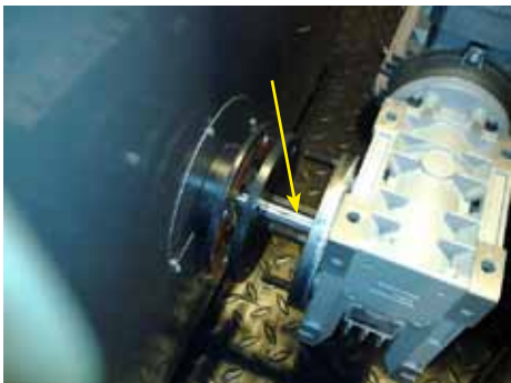
Insert the motor into the primary screw shaft.
