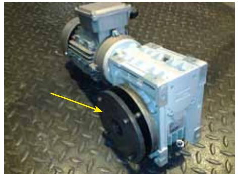
Install the ash screw adapter flange onto the motor adapter flange.
