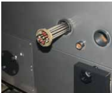
1. Installation of the resistance
