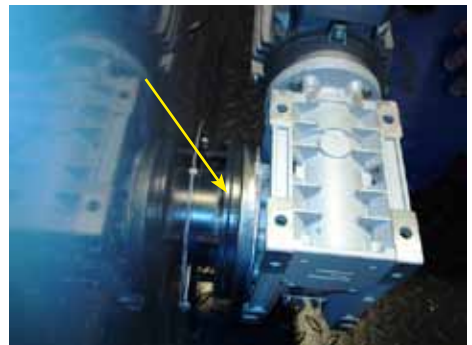
Push the motor into the mounting flange.
