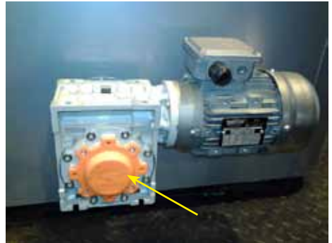
Install the bearing cover plate.
