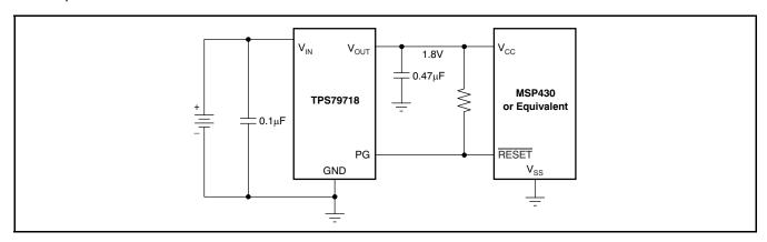
Figure 15. MSP430 Microcontroller Powered by the TPS79718 Regulator
