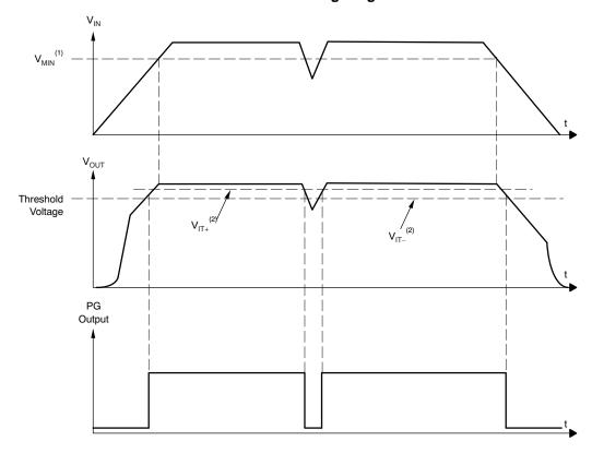
NOTES: (1)  $V_{MIN} = V_{OUT} + V_{DO}$ . (2) The PG trip voltage is typically 10% lower than the output voltage (90%  $V_{O}$ ).  $V_{IT+}$  to  $V_{IT-}$  is the hysteresis voltage.
