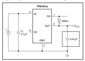
Figure 14. Typical Application Circuit
