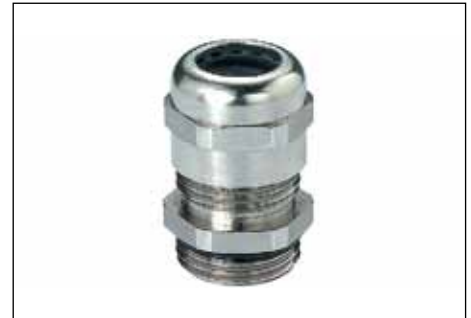
MEMV: – Metric – IP 68, 5 bar (30 min.) / DIN EN 60529 – Brass, nickel-plated – Integrated strain relief – Anti-twist protection – Temperature range: -20°C to +100°C – For leads with shielding – Fast, easy EMC connection of the screen mesh via the contact spring and the intermediate connection with the enclosure potential. – The protective shield is permanently formclosed over a large area of the enclosure
