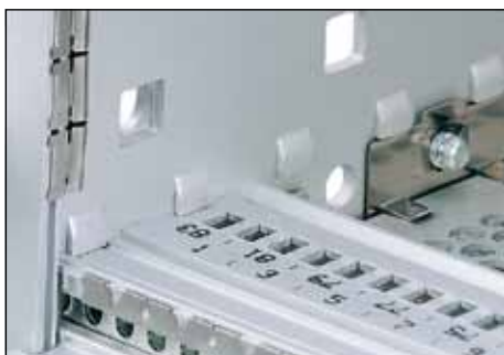
Torx screws hold the profiles in position. When turned, they are automatically pressed against the protruding boss, secured against turning, and positioned exactly.
