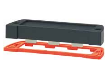
ASD – The end cover is equipped with a 2 mm recessed area for fitting membrane keypads. All lids are fitted with contact areas which contact the lid to the profile. This guarantees good EMC protection even for the standard enclosure. Black metal-filled EMC seals are available for increased EMC resistance.
