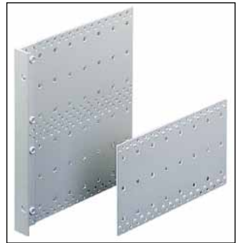
Side panels in 2 versions, 5 different heights and 6 different depths. For extreme mechanical loads, the support brackets are firmly riveted to the side panel. All side panels are passivated, so have a conductive function.
