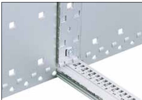
A shielded backplane is screened against the side panel by means of a vertical profile with a fitted EMC spring.
