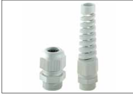
BF / MBF / BFK / MBFK: – Pg/Metric – IP 68, 5 bar (30 min.) / DIN EN 60529 – Polyamide, light grey, similar to RAL 7035 – Integrated strain relief – Temperature range: -20°C to +100°C – VDE certificate (MBF only): no. 134176 – Integrated anti-kink protection (BFK/MBFK)
