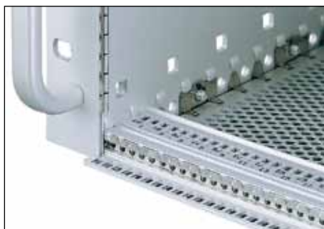
EMC springs are clipped onto a conductive area of the profiles; the subracks provide the necessary contact to the screened front panel.
