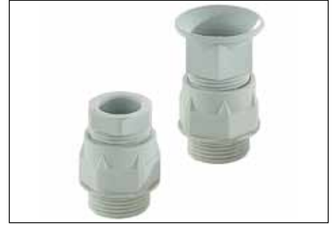
POZ / MPOZ / POZB / MPOZB: – Pg/Metric – IP 65 / DIN EN 60529 – Polyamide, light grey, similar to RAL 7035 – Integrated strain relief – Temperature range: -30°C to +100°C – Integrated anti-kink protection (POZB/ MPOZB)
