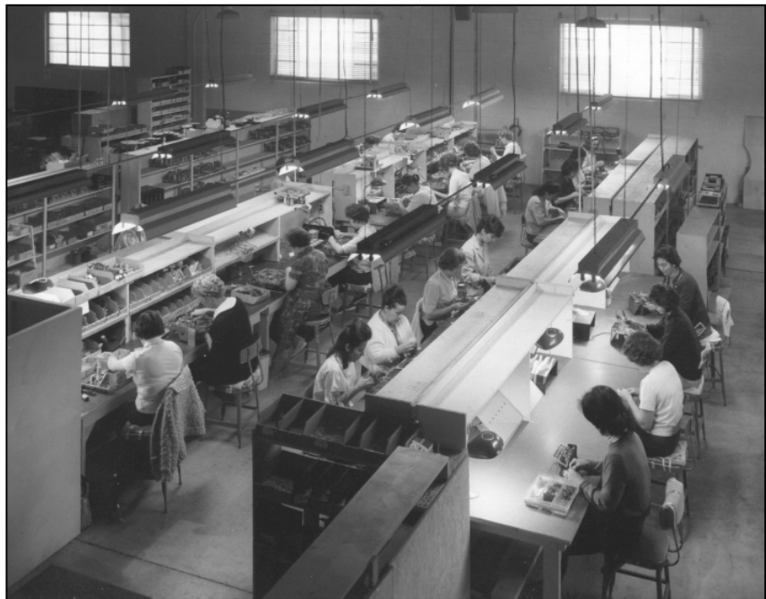
Figure 1-4 Primary Component Wiring Area
