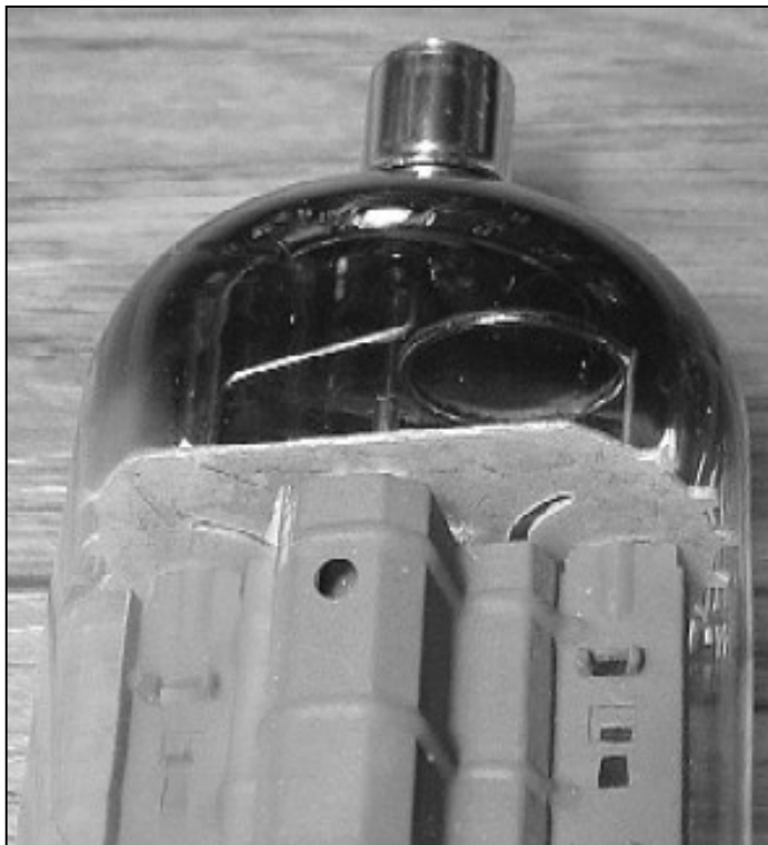
Figure 8-2 Getter Placement Example (6MJ6)
