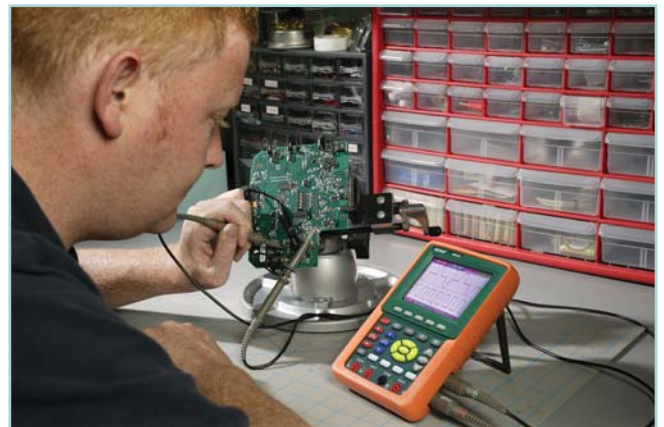
Dual trace testing or troubleshooting of printed circuit boards and electronic assemblies
