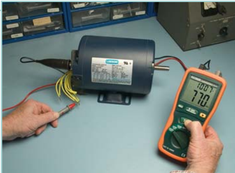
Measures the insulation resistance of motors.
