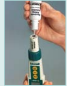
Unique gel filled or refillable (pictured) flat surface electrode design
