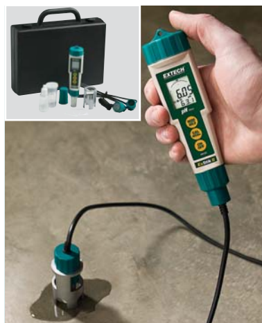
Measure pH level of concrete using a pH meter with a flat surface pH electrode plus a metal weight probe guard for stability and protection
