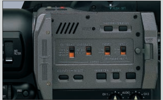
Sub-panel (with LCD monitor opened)
