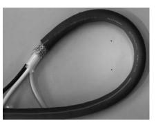
•Lead-free mixed vinyl, which is flexible and oil and heat resistant, is used for the sheath. The cable can be used for high-speed transmission at 10 Mbps and helps the CC-Link display full performance. The transmission distance is 50% of that of the standard cable. (Example: Max. 50m at 10Mbps) •The standard cable length is 100 meters.
