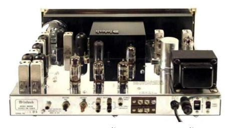
**BACK PANEL:** TP 2 scope output. MUTING adjustment. OUTPUT adjustment. AUDIO OUTPUTS 2.5V fixed and FRONT PANEL CONTROLLED. EXT STEREO INPUT. Screw terminals for 300 or 75 ohm FM ANTENNA and TO TV SET. Power cord. FUSE. Unswitched AC outlet. PANEL LIGHT switch: BRIGHT or DIM.
