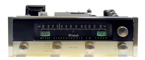
FRONT PANEL: Anodized gold and black aluminum panel. Illuminated dial. Illuminated SIGNAL STRENGTH meter. MPX indicator light. Illuminated TUNING meter. Tuning control. VOLUME control. MODE SELECTOR switch: EXT STEREO, MPX STEREO, FM, POWER OFF. AUTO FREQuency control: MIN to MAX. MUTING switch: IN or OUT. ZERO ADJUSTMENT for signal strength and tuning meters behind end caps.
