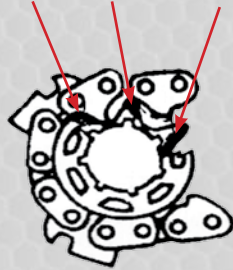
Chain cannot mesh cleanly with sprocket
