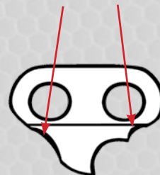
Wear on front and back of drive links
