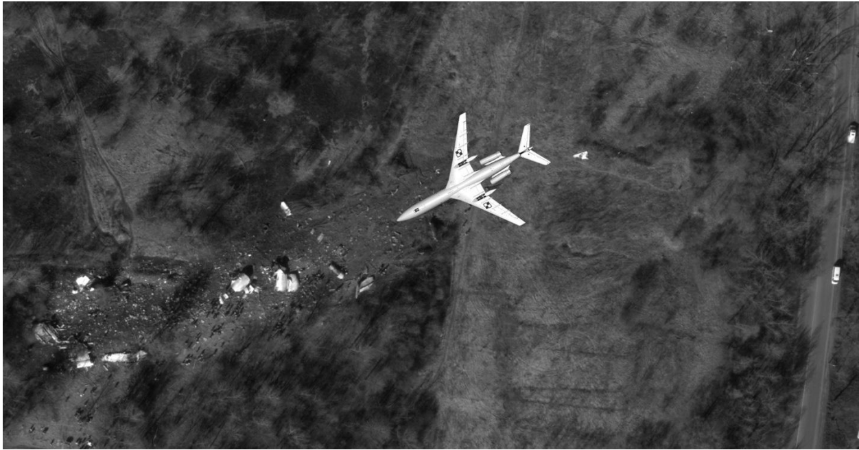
Fig. 35. A view of the crash site compared to TU154M in reverse position in correct scale.
