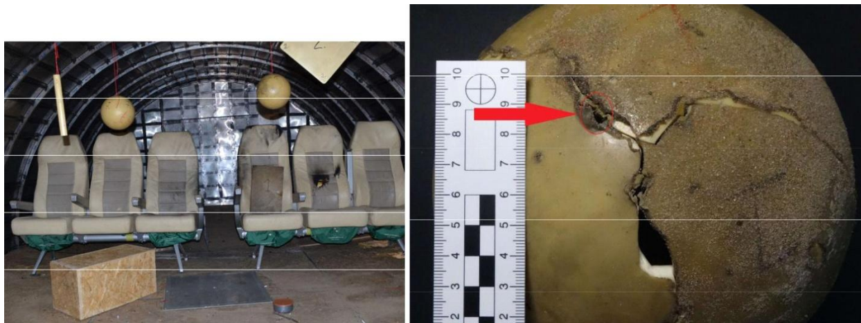
Fig. 53 Medical phantoms inside the model of the aircraft cabin.
