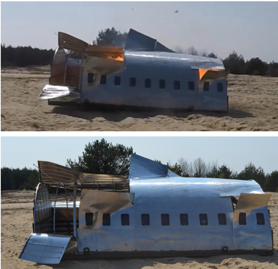
Fig.51. The outcome of an explosion of jet-fuel in the cabin of the fuselage resulting in a large opening but no destruction into small pieces.
