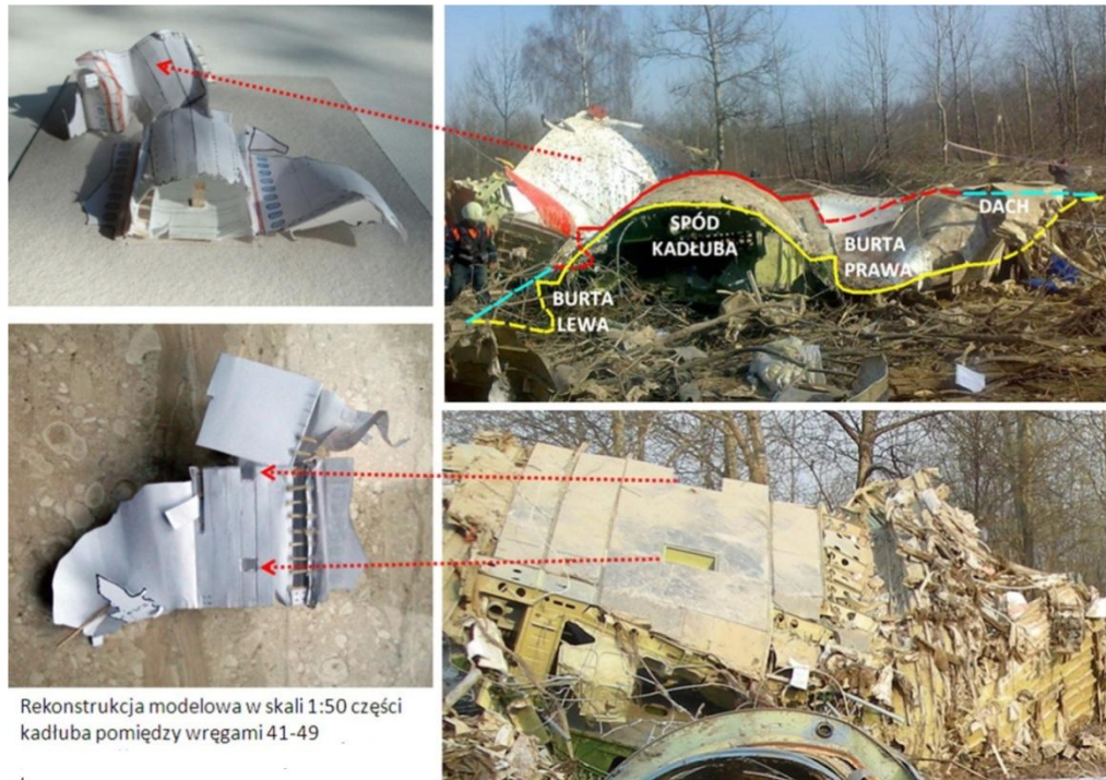
Fig. 44. Image of the fuselage destruction with both sides of the fuselage opened and thrown outwards.
