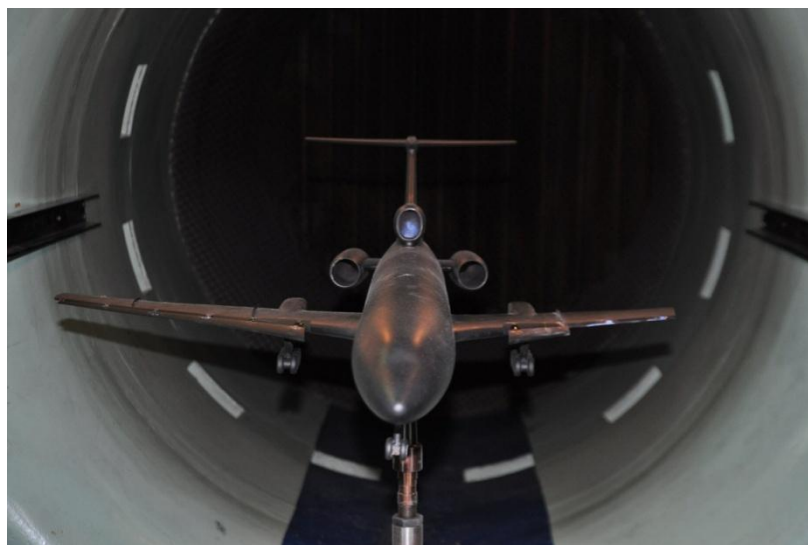
Fig. 25. Airplane model in the wind tunnel of the Institute of Aviation. This version includes a cut left wing and is without slats and the outer flap.
