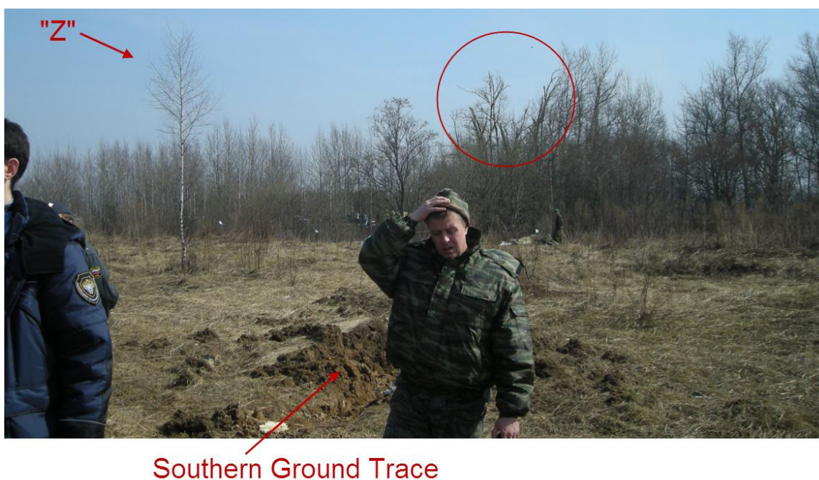
Fig. 31a. The tree marked "Z" growing in the direct vicinity of the flight path, where the plane flew from Kutuzov Street (red circle) to the place of crash. The ground trace from the tail is visible and marked here as "Southern Ground Trace".
