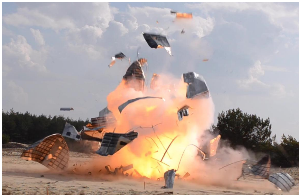
Fig. 52 The outcome of an explosion of a thermo-baric charge in the cabin of the fuselage resulting in the complete destruction of the fuselage and the formation of a large quantity of small debris.
