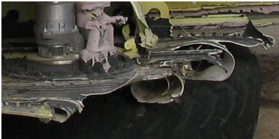
Fig. 2. Side view of the broken section of the left wing tip of the TU-154M no.101 showing significant explosive signatures (curled edges of up to 450°).
