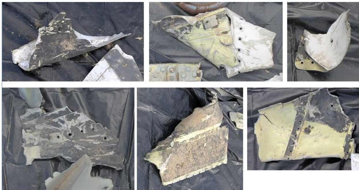
Fig. 10. Fragments of the bottom skin curled outside the structure.
