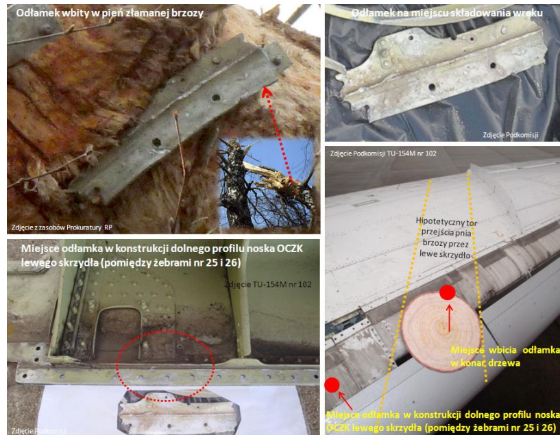
Fig. 5. The place in the wing construction of the piece rammed into the so called Bodin birch tree.
