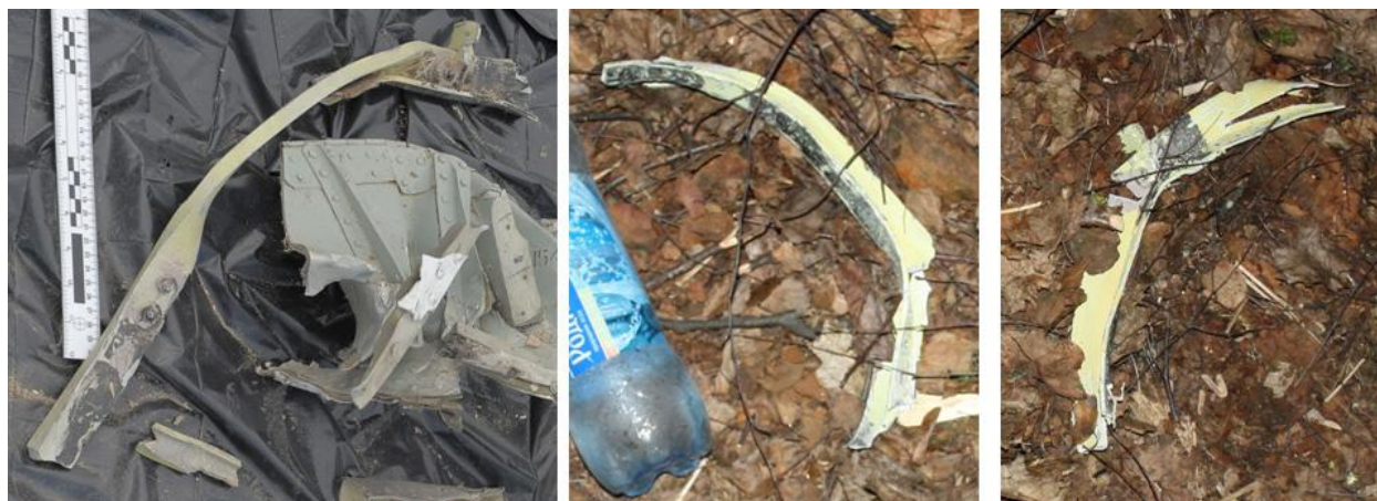
Fig.8. Pieces of stringers of the left wing curled outwards
