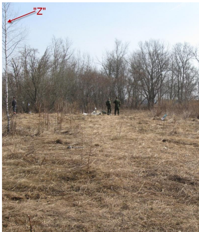
Fig. 30. The tree marked "Z" growing in the direct vicinity of the flight path, where the plane was flying from Kutuzov Street (in the background) to the place of the crash. On the right side, starting at the blue marker on a tall stem, there is a visible trace in the ground, where the left stabilizer ploughed through.
