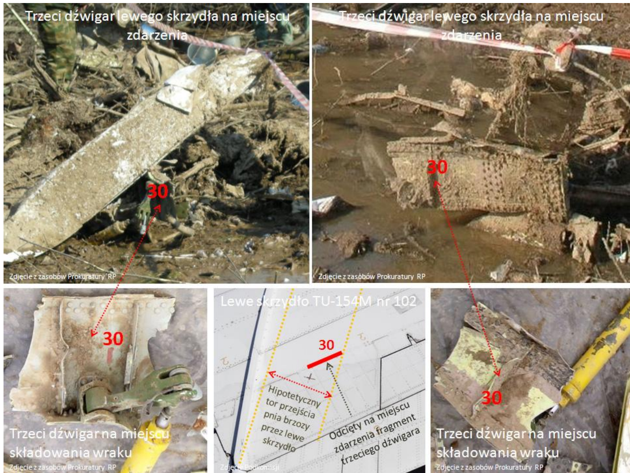
Fig. 15. View of the same part of spar no.3 from the detachable part of the left wing on the main crash site (top two pictures) and place of storage of the debris (bottom left and right pictures). The bottom middle picture is a drawing of the left wing of TU-154M, No. 102, where the red arrows show the hypothetical trail of the 'bb tree' through the left wing, while the black arrow shows the location of the part of the third spar.
