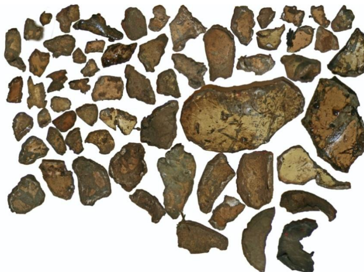
Fig. 33. Collected pieces of the Tu-154M taken from the ground 100m before the main crash site, having visibly undergone thermal change.
