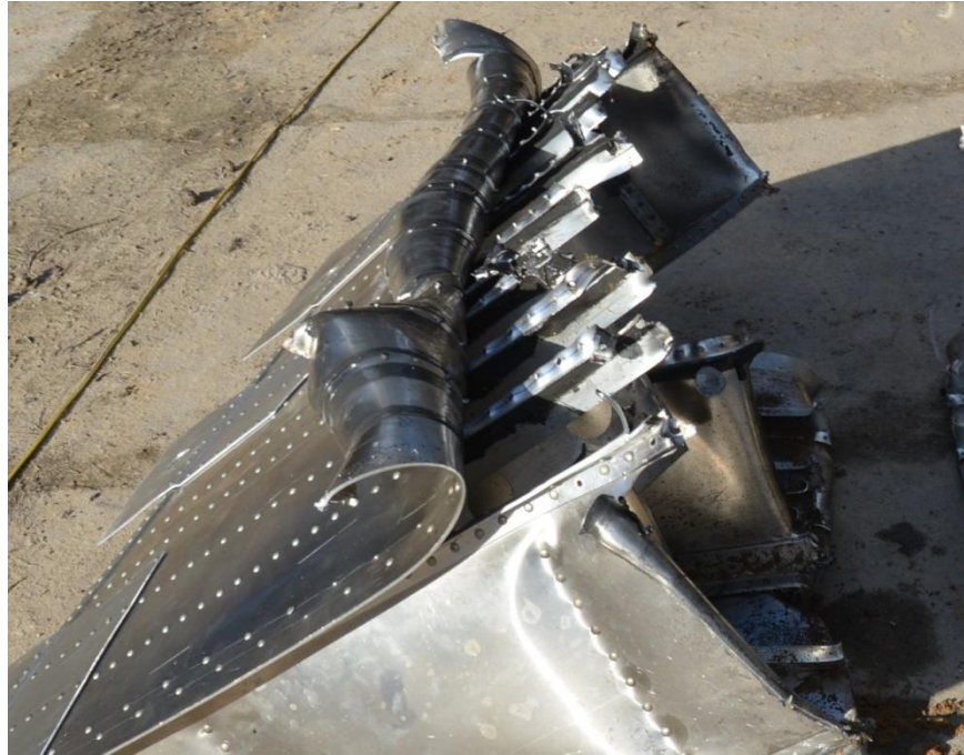
Fig. 23. Separation by explosive material of the wing box containing fuel (Scale 1:1). The experiment demonstrated the wing could be cut (destroyed?-) without a secondary, major fuel explosion.
