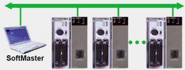
Remote connection using Ethernet
