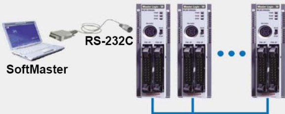
Remote connection using RS-485 Communication
