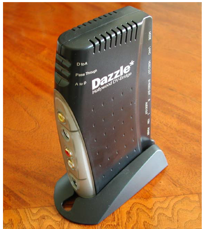
FIG. 1: The Dazzle Hollywood DV-Bridge is a compact converter for importing video into, and exporting video out of, a personal computer. The unit sells for $299.99.
