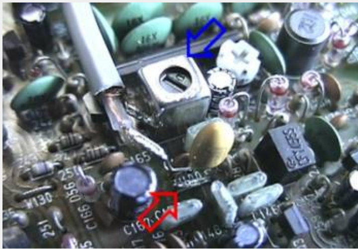
The red arrows indicate the location of wire link "W100" to which a 10u capacitor is soldered The blue arrows indicate the location of the metal can to which the shield from the audio cable is soldered
