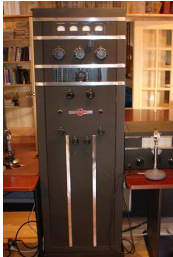
1946 – 30K-1 AM/CW transmitter. Input power 500 watts CW, 375 watts AM, 80-10 meters. Price $1450, included 310-A exciter
