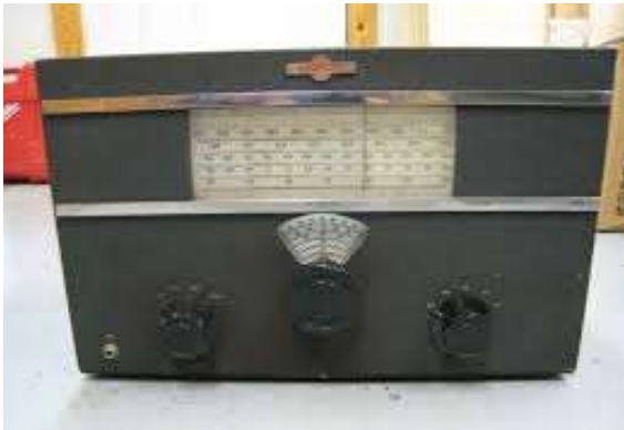
1946 - 310A used the 70E-8 PTO with an AC power supply. PTO/Exciter for 30K-1 transmitter. $100
