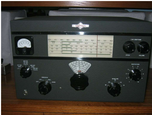
1949 - 310A-3 powered from 30K-1 and used as PTO/exciter for 30K-1 transmitter
