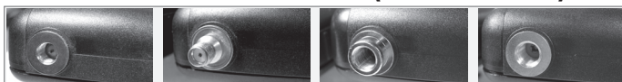
A (SMA M) B (SMA F) C (MX F) D (M/A COM F)
