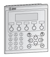
The **E50** is a key-oriented HMI unit with four function keys and an LCD display with two rows and 16 characters each. It can display up to 50 text blocks, which can be paged with the function keys. Values can be edited directly with the unit's keyboard. The RS232C and RS422 ports are both integrated in a 25-pin connector.
