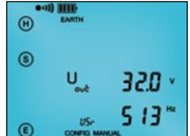
The Frequency selection screen displays selected test frequency and voltage for the test as well as lead connection.
