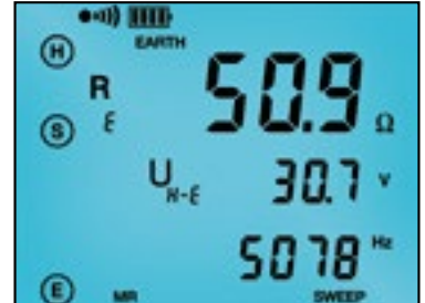
The 3-Point Fall-of-Potential test displays test lead connection, grounding electrode resistance, test voltage and frequency.
