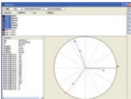
Display real-time Phasor diagrams. Includes unbalance for both voltage and current.
