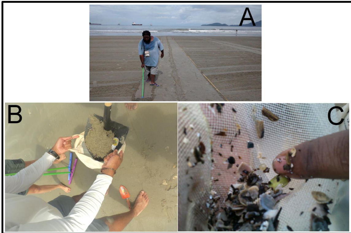
Figure 6. Sampling procedure. A: Pushing of the plastic pellets present in the intertidal zone with a squeegee. B: Accommodation of the detached sediment in the 0.1 mm sieve for posterior washing. C: Washed material containing plastic pellets.
