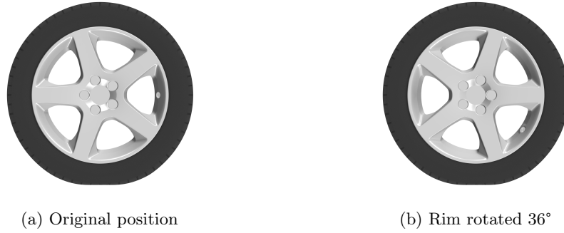
Figure 1.2: Different positions for the rim, resulting in different solutions when using MRF.
