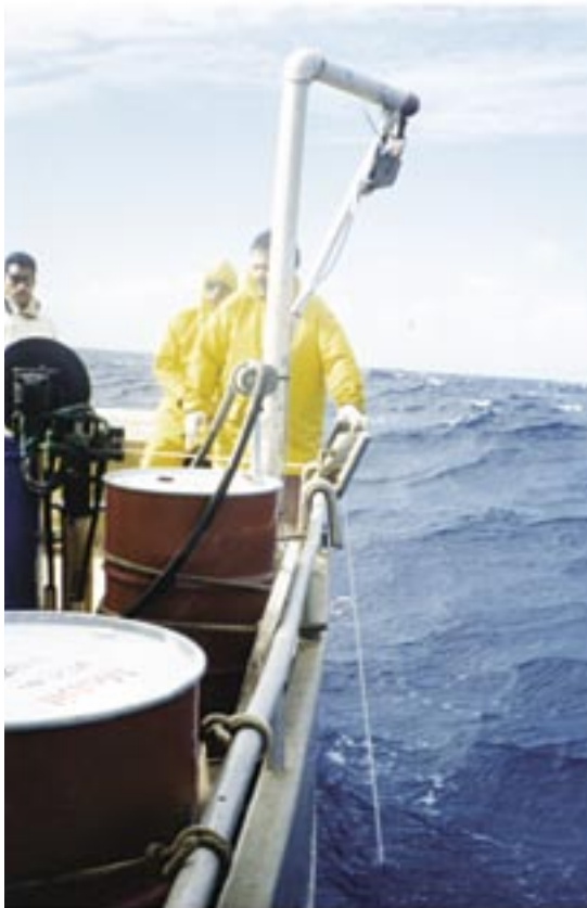
FIGURE 19 One type of line hauler used to haul bottom longline
