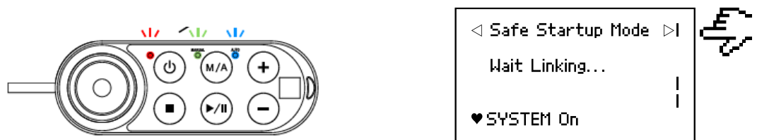
Figure 2: The Three Lights on The Robot Stick Flashing
