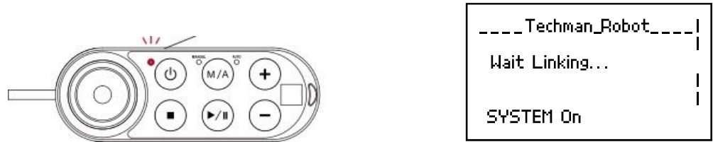
Figure 9: The Power Light on The Robot Stick Flashing
