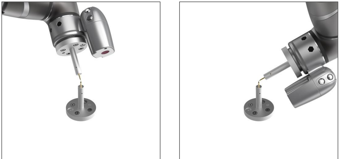
Figure 103: The Robot Posture Needs to Change during Teaching (1/2)
