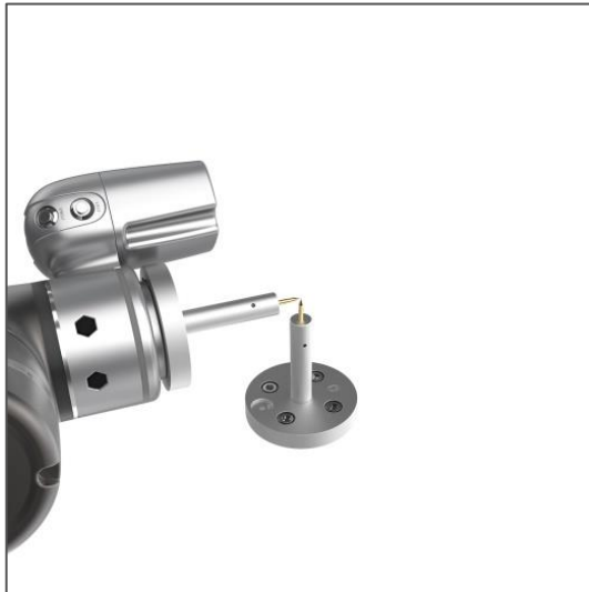
Figure 104: The Robot Posture Needs to Change during Teaching (1/2)
