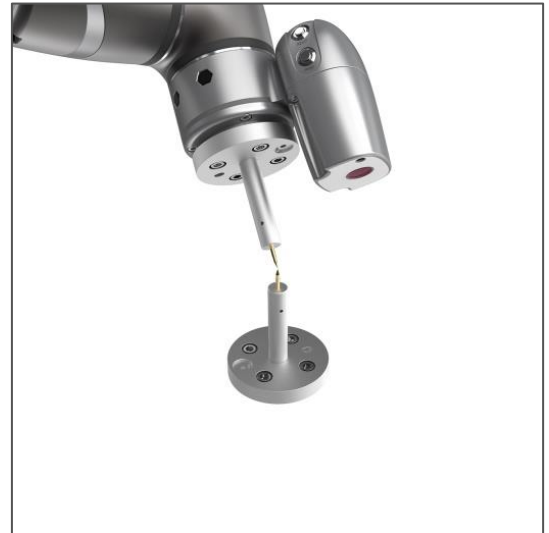
Figure 104: The Robot Posture Needs to Change during Teaching (1/2)
