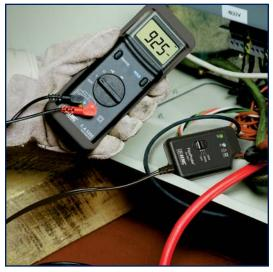
FlexProbe<sup>®</sup> conveniently plugs into the standard DMM voltage input for direct read-out of the measured current.
