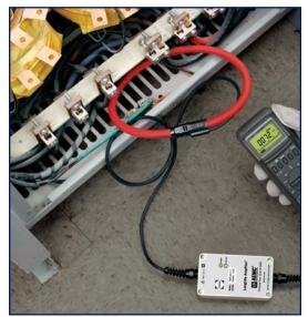
Model LGLF 1000-24-1-1 measuring on one phase of the primary side of an in-plant three-phase transformer.
