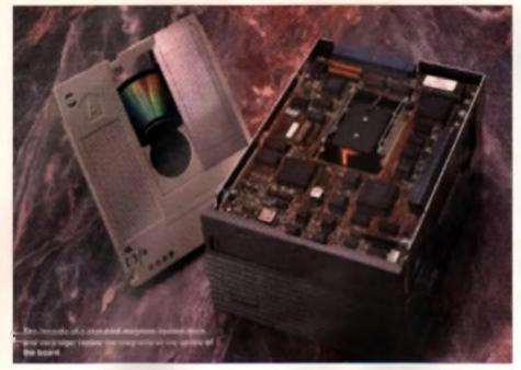
netcally alterable if room temperature, but only when heated up. Writing data to this type of disk requires both a magnitude write head and a laser, which is focused on a tiny area of the disk which then heats up to the required temperature to change. As the laser can locus extremely accurately, the area actually changed by the magnet is tiny, so you can get 128Mb of data into a cartridge only a little larger than a 3.5° disk.
