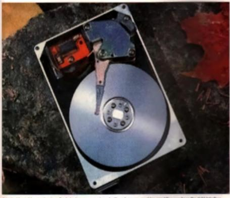
A typical bare drive mechanism. Such devices are generic and will work on any machine providing you have the right interface
