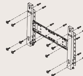
Check the installation diagram and mark the drill points on the wall. Use the 5.0 mm bit to drill holes deeper than 35 mm. Fix each anchor in the corresponding hole. Match each of the brackets and hinge holes to the corresponding anchor holes and insert and tighten the 11 A screws.
