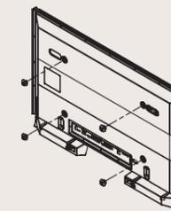
Remove the 4 screws on the back of the product. Insert screw B into the plastic hanger.
