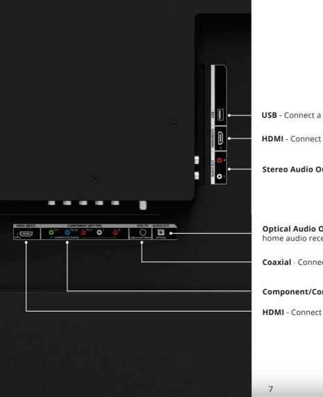
**USB** - Connect a USB thumb drive to display photos.
