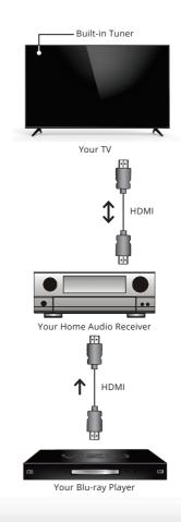
With an HDMI ARC setup, the audio connection between your TV and home audio receiver can be removed. The HDMI cable will transmit audio signal to and from your TV with an all-digital audio/video connection.
