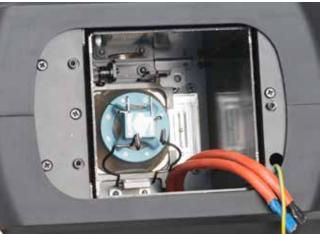
6. Using two fingers, gently remove old lamp from the fixture. (See below)
