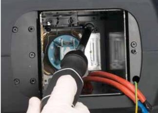
10. Gently attach (2) Wires to spade terminals on the base of the lamp. (See below)
