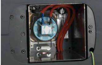
11. Replace lamp cover and secure (3) screws marked "A", "B", and "C". (See below)
