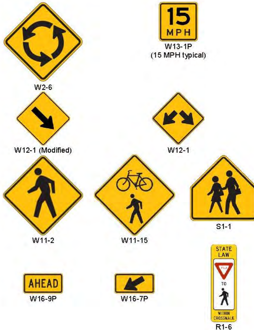
Figure 4.09.6.02.1 Roundabout Warning Signage
