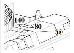
Round trays for both 80 slides and 140 slides can be used. The tray setting switch (10) is set in the factory to accommodate the 80 tray. By using a small screwdriver, the switch can be brought into the 140 position.
