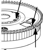
1 • Check that the baseplate of the slide tray is locked into zero-position and cannot be rotated.
