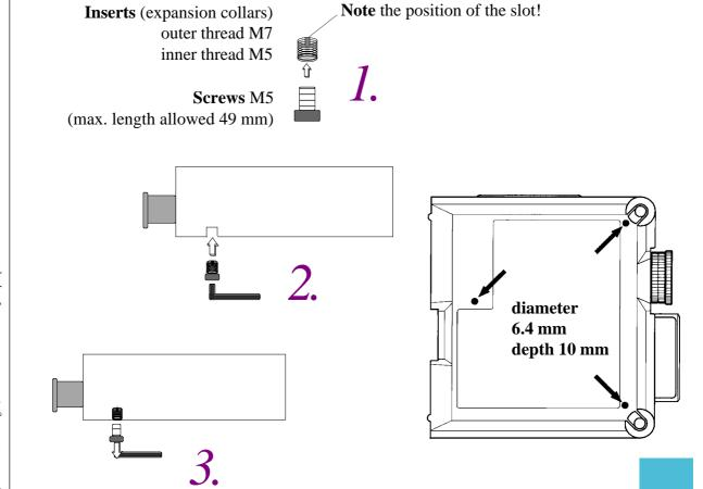
Compliments of: Professional Installation **Fixing Holes Fixing Holes** diameter 6.4 mm depth 10 mm 38,00 106,00 50,00 204,00 63,50 40,00 38,00 52,00 250,00 40,00
