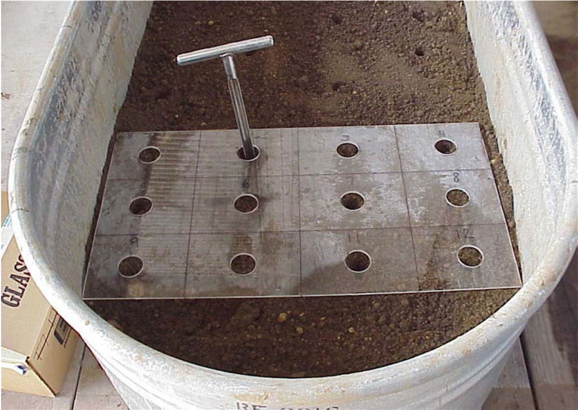
Figure 16. Photograph of sampling grid and soil corer used to collect samples from the troughs
