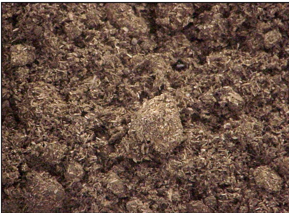
Figure 13. Change in soil texture following addition of the rice hulls as bulking agent
