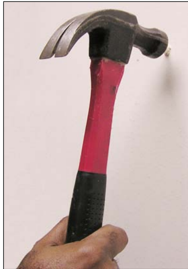
Figure 2.10 Hammering Plastic Anchors
