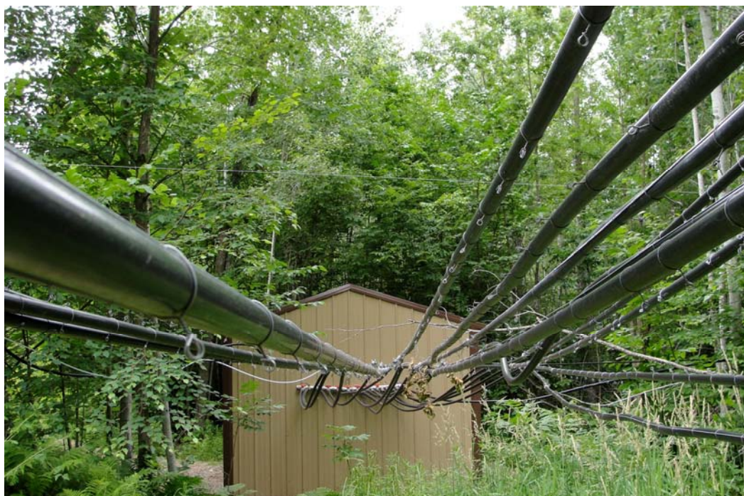
Multiple sap lines running from the sugar bush into the Timber Sweet pump house, a vacuum-tap commercial operation. Photo by D. Wilsey.
