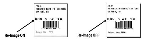
In the above example, Option 61 was applied to the bar code field to keep the incrementing field (Box #) from blocking out the bar code field.
