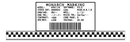
The test label shows the model number, software version, total number of inches printed, voltage, print contrast, printhead resistance, code page, MPCL control characters, ENQ and RS232 characters.
