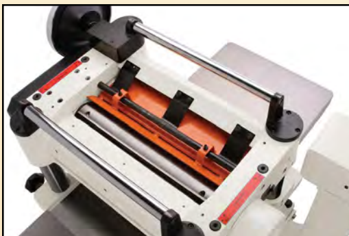
W1742 Cutterhead & Triple Springs on Chip Breaker
