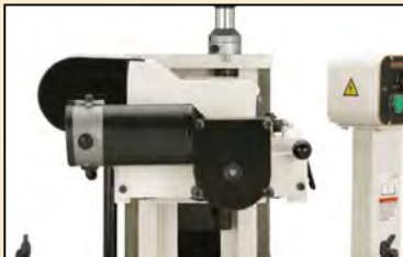
Open-Sided Cutterhead Assembly Travels on Dovetailed Column Way
