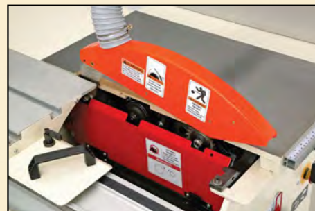
Blade Guard with Dust Port, Riving Knife and Scoring Blade
