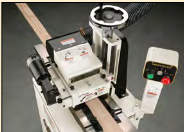
Efficient Chip Collection w/ Cutterhead Viewing Window
