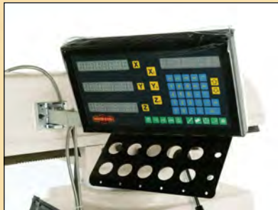
3-Axis Digital Readout with Collet Tray
