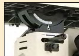
Heavy Cast Iron Trunnion & Quick Lock Table
