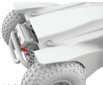
Figure 4.6a Extreme X8 brake levers engaged
