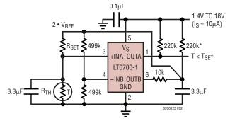
$R_{TH}$  = 1M (e.g., YSI 44015, 1.00M $\Omega$  AT 25°C)  $R_{SET}$  =  $R_{TH}$  AT  $T_{SET}$  \*RESISTANCE MAY REQUIRE OPTIMIZATION FOR OPERATION OVER INTENDED  $R_{TH}$  AND  $V_{SUPPLY}$  RANGES HYSTERESIS ZONE  $\approx 0.4$ °C
