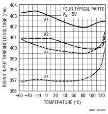
**Rising Input Threshold Voltage** vs Temperature
