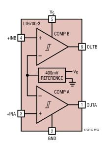
**OUTA (Pin 1):** Open-Collector Output of Comparator Section A. This pin provides drive for up to 40mA of load current. Off-state voltage may be as high as 18V above GND (Pin 2), regardless of  $V_S$  used.
