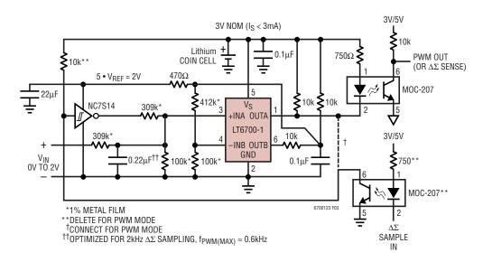
Figure 3. Isolated PWM or  $\Delta\Sigma$  Converter
