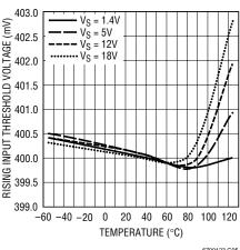
**Rising Input Threshold Voltage** vs Supply Voltage
