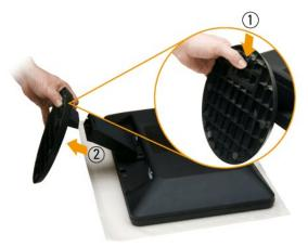
After placing the monitor panel on a soft cloth or cushion, complete the following steps to remove the base.
