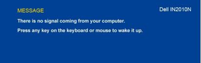
If VGA input is selected and VGA cable is not connected, a floating dialog box as shown below appears.
