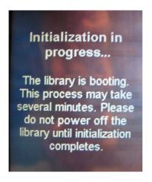
**Caution:** From this point forward until the process is complete, do NOT remove power from the library! Doing so may cause failure and cause LCB to become unusable.
