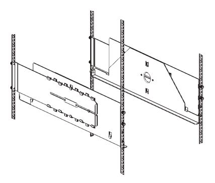
**f** If the studs do not reach the mounting holes, pull the front of the shelf toward you to extend it to the necessary length. Hold the base of the shelf with one hand, and pull the extensible part of the shelf with your other hand.
