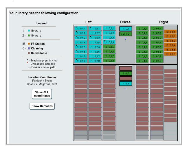
**8** If a partition references tape drives within the module you are removing or replacing, modify any affected partition by removing the referenced drive elements from the partition. See <a href="Modifying Partitions">Modifying Partitions</a> on page 75.
