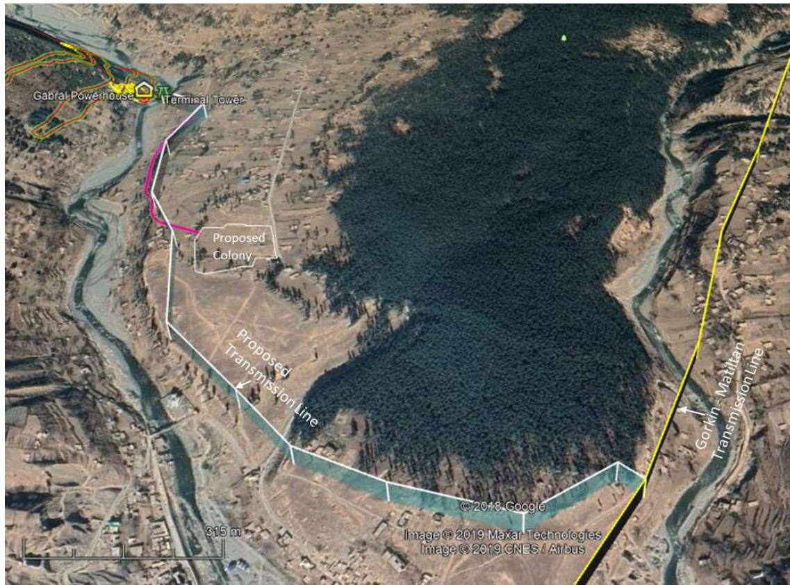
Figure 3.6: Proposed Alignment of the Transmission Line
