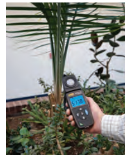
Measure and record multiple measurements to create an illuminance map of the room or area of interest
