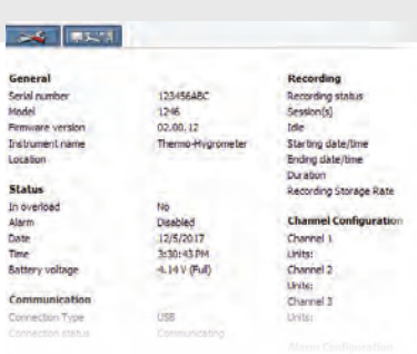
Typical status screen shows current state of the instrument
