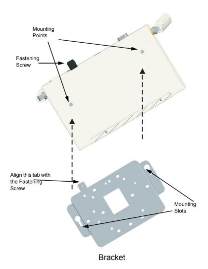
lines up with the tab on the bracket. Then screw down the fastening screw to secure the access point to the bracket.
