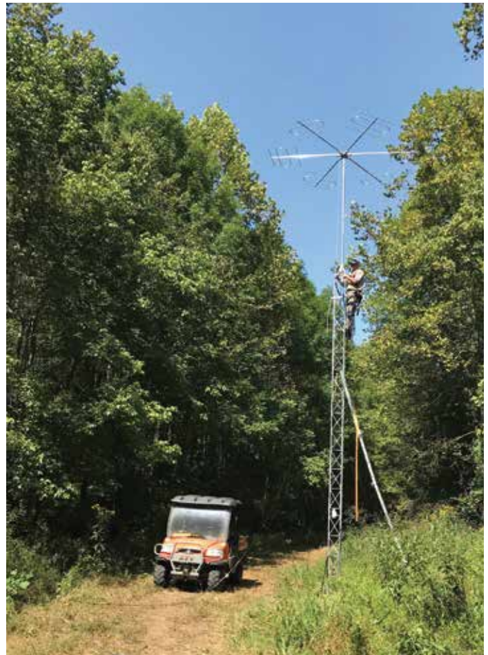
This automatic telemetry system installed at Yellowbank WMA helps detect the presence of Indiana bats. Photo: KDFWR
