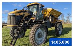
**2014 AGCO RG1300 RoGator**, 1892 hours, AGCO 8.4L 330 hp turbo diesel engine, 4WS, painted 409 SS New Leader L4000G4, Raven Viper Pro, Phoenix 300 GPS, parallel swathing, air ride seat, A/C, beacon lights, fenders, electric roll tarp, Michelin 380/90R46 tires (front 45%, rear 35% remains).
