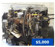
2010 4660 SpraCoupe Perkins Diesel Engine 1104D, 874 hours, 4 cylinder, 4.4L (269 in.3), 125 hp (93 kW) at 2200 rpm. Engine includes: alternator, starter injection pump, turbo charger, and primary fuel filter and housing. (PA)
