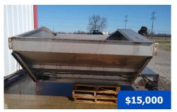
**2017 Double Duty 7' Insert,** 7 ft multi-product insert, fits in 13 ft spreader body, 304 SS. All electrical and hydraulic connections included.
