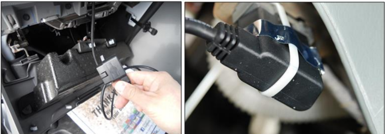
Figure 10: Plug Male Connector of OBD-II Extender Cable into OBD-II port.
