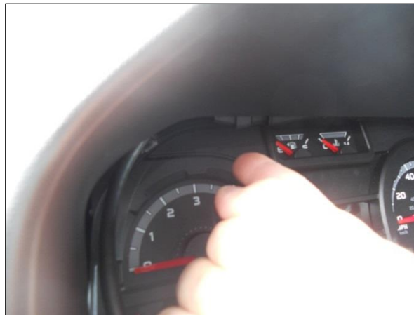
Figure 12: Tuck LMU-30xx/CVF-3030 Behind Panel
