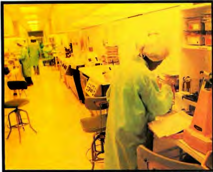
Photo 1: Processing. Photosensitized wafers are exposed with a particular mask pattern using ultraviolet light. The entire environment is otherwise ultraviolet-free.
