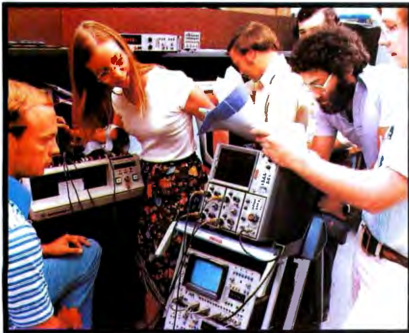
Photo 2: Breadboard debug. The gate level TTL model of the processor involves ten boards of 80 to 120 integrated circuits each. Many of the required 10,000 connections will be wrong. The system must be tested to find and correct construction and logic errors.
