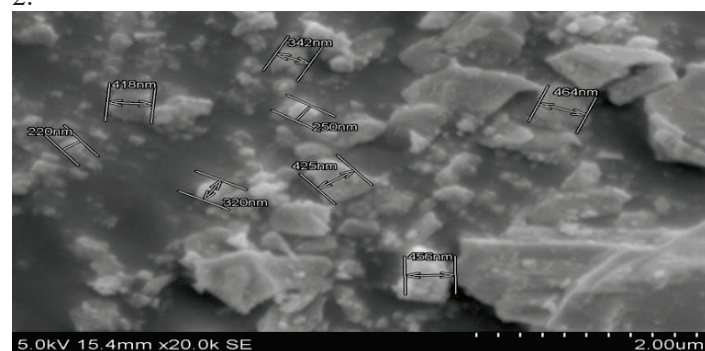
Figure.1. SEM image of manganese dioxide powder
