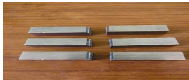
FIGURE V: Broken standard DSS specimen
