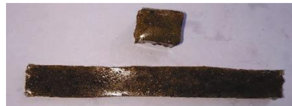
Figure 2. Specimen manufactured using hand layup technique
