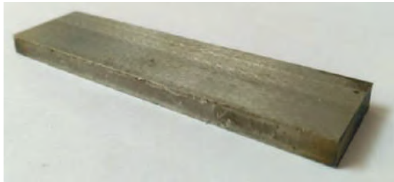
Figure 3.6 Inconel 718 workpiece 100 x 27 x 5 mm (iso)
