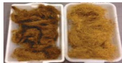
Fig 4(a): Brown and white coir fiber after sodium hydroxide treatment
