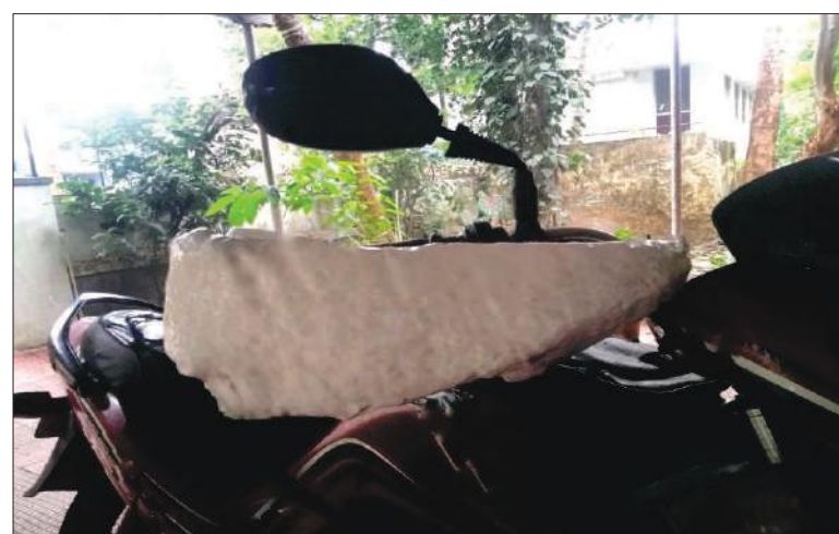
Figure 3.9: Cross woven bamboo fiber reinforced epoxy composite, Hand guard installed in a bike
