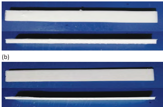
Figure 5. Sample printed using FDM (a) impact model (b) tensile model
