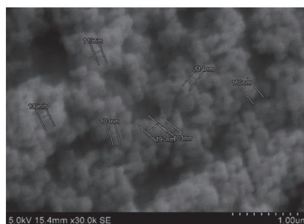
Fig. 1. SEM image of titanium dioxide powder
