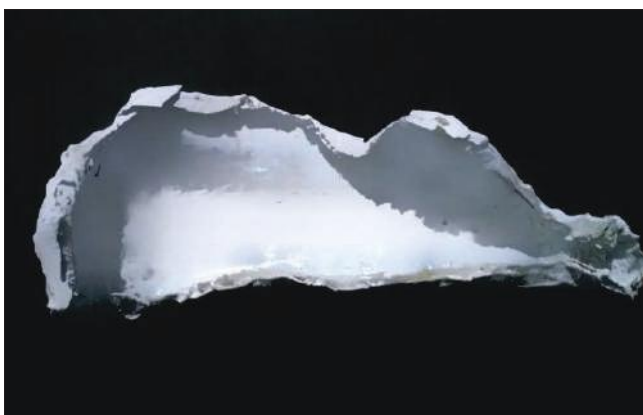
Figure 3.6: Mould –made up of plaster of paris
