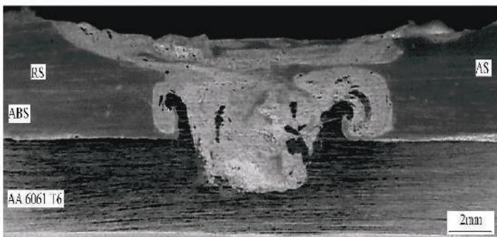
Fig. 6 Cross-sectional view of joint welded at 500 rpm tool rotation, 14 mm/min feed rate and 20 mm shoulder diameter.
