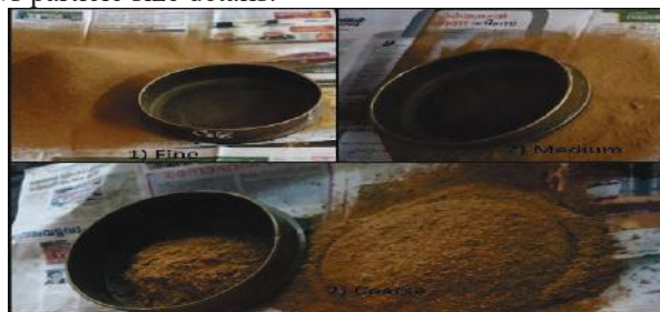
Figure 1. Wood particle of particle size fine, medium and coarse
