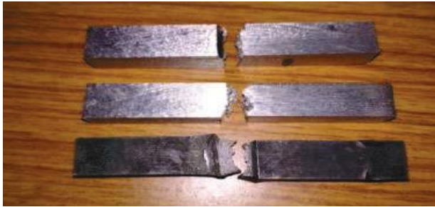
FIGURE VXI: Broken niobium stabilized DSS specimen
