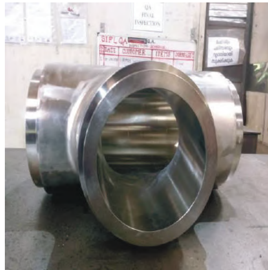
Fig 3: Trepanned Ti6Al4V T block
