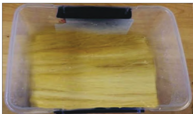
Figure 1.3 Bamboo fiber soaked in 6% NaOH solution
