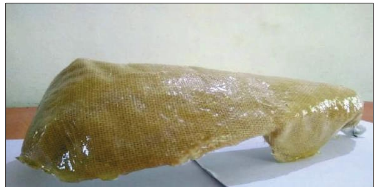
Figure 3.7: product (hand guard for bikes-cross Woven bamboo fiber reinforced epoxy composite)
