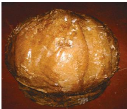
Figure 17. Industrial safety helmet manufactured from wood powder composite
