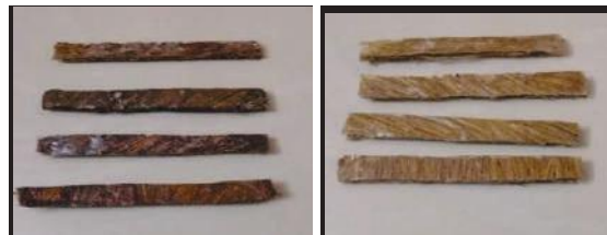
Fig 4(b) and 4(c) brown and white coir treated reinforced polymer composites with 90,30,60,0 respectively
