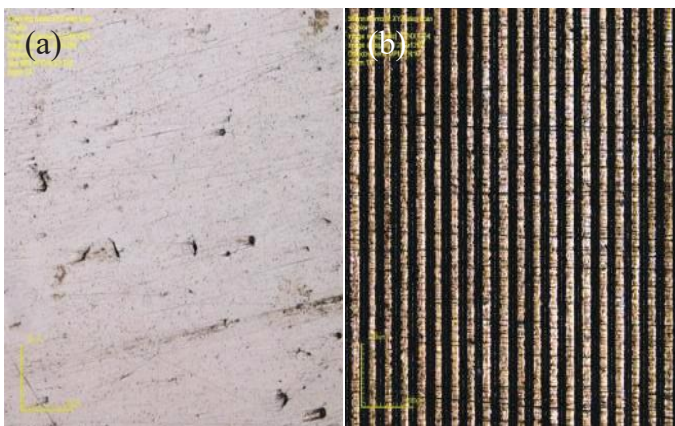
Fig.3Wetting of water in (a) Polished and (b) Textured Titanium grade-5
