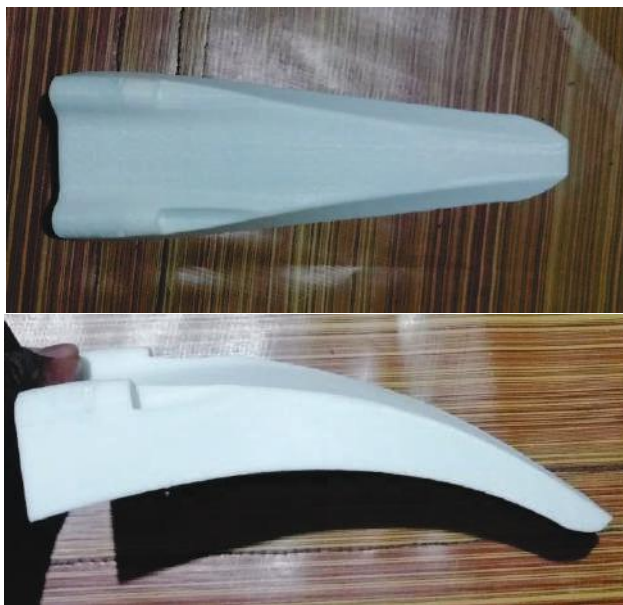
Figure 8. FDM Fabricated ABS Fender
