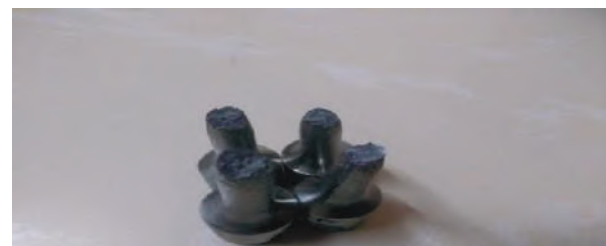
FIGURE I: Broken tensile test specimen
