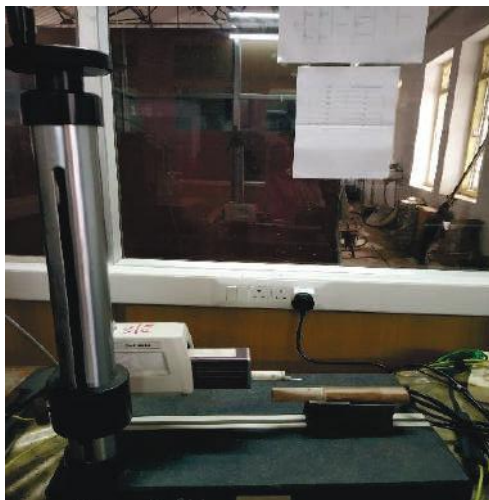
Figure 5. Specimen on which turning operation performed and apparatus by which surface roughness measured (using Profilometer)
