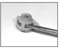
By inserting a small screw driver between the valve seat (27) and the valve spring retainer (30), the valve assembly can be separated.
