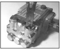
Using a needle nose pliers, remove the inlet and discharge valve assemblies (27-30) and o-ring (31). Inspect all parts for wear and replace as necessary.
