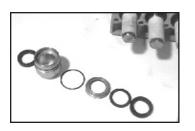
Remove the weep return ring (25), pressure ring (24), and v-sleeve (23) from the valve casing (26). Remove the rear v-sleeve (23A) from the seal case (20). Inspect pressure ring (24) behind the seal case (20).Inspect all parts, including o-ring (21) for wear and replace as necessary.
