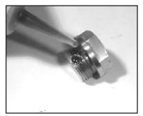
Remove the o-ring (31) Inspect all parts for wear. Apply one drop of Loctite 243 to the valve plugs (32) and tighten to 55 ft.-lbs. (75 NM).
