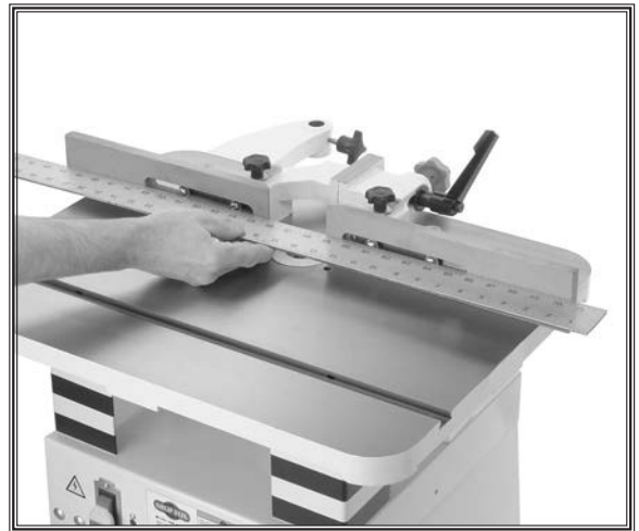
Figure 21. Use straightedge to check fence.
