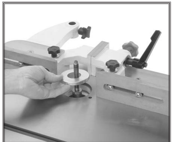
Figure 22. Using table insert to keep wood shavings on the table.
