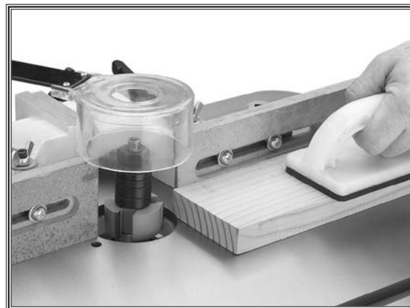
Figure 15. Shaper cutter installed on spindle.
