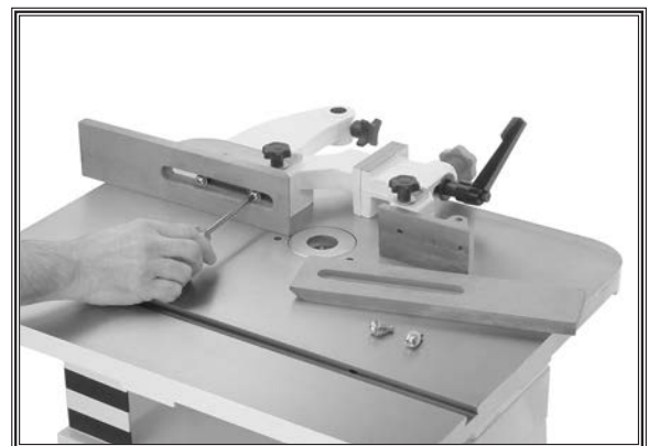
Figure 10. Installing fence facing.
