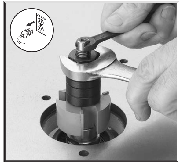
Figure 27. Tightening spindle nut.
