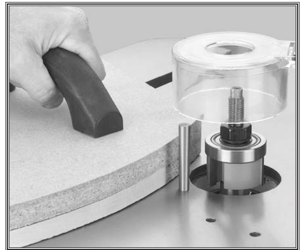
Figure 36. Using a starting pin with a hold-down jig to support workpiece.
