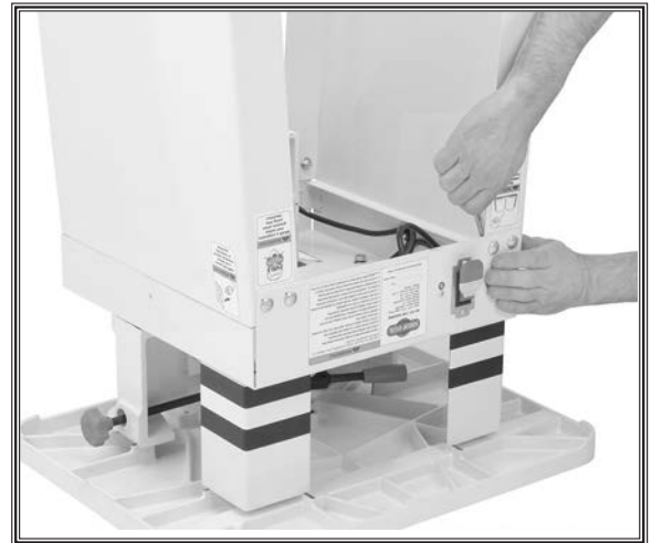
Figure 9. Attaching stand to shaper unit.
