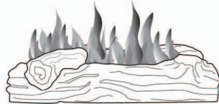
Figure 11 - Incorrect Burner Flame Pattern (Excessive flame height, combined with extremely yellow flames producing carbon (soot)).
