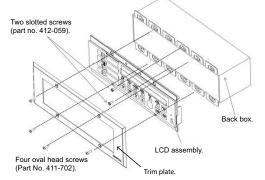
Figure 6. Expanded view of 4603-9101 LCD Annunciator
